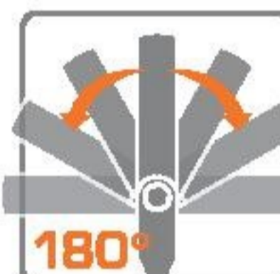
180° flex head has 13 Locking Positions.
