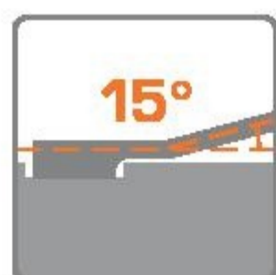
15° Offset Box End helps to reduce swing obstacles and to minimize knuckle fatigue.
